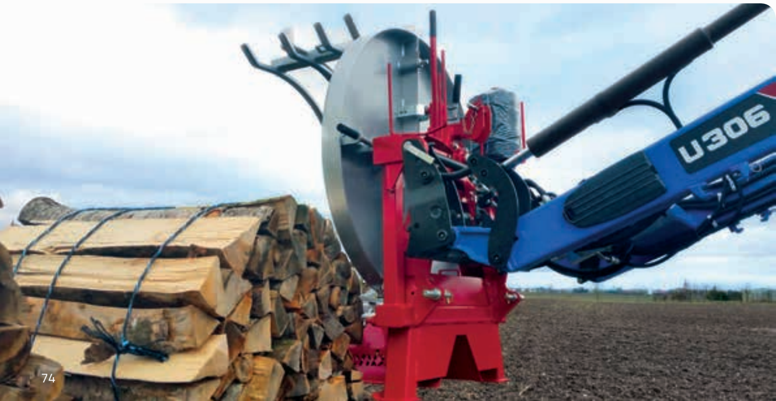
Bundler with polyester strips mechanical pivoting on 3-points hitch + euro linkage for front loader
