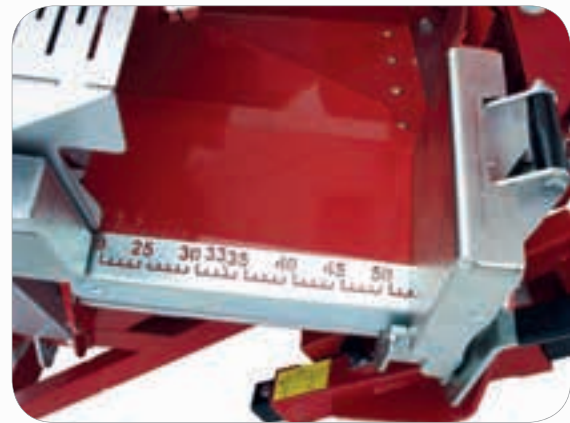
Set the cutting length of 20-52 cm with a notch lever
