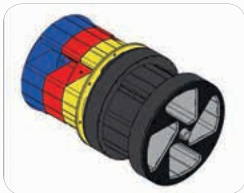
A drum in 3 parts The internal part is made up of 3 telescopic parts in order to guide the wood along the drum
