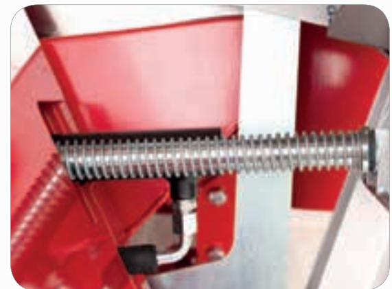
Hydraulic log carriage system
