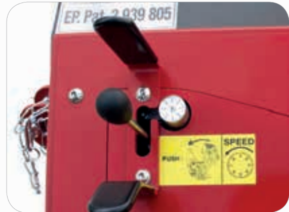
Valve and speed regulation for log carriage
